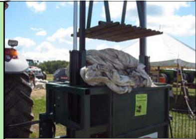
"BigFoot" agricultural plastics baler. This machine makes 1,000 pound bales which can be recycled!
